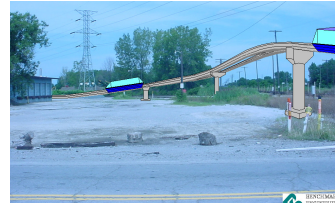
MULTI-Freight Beams slope up eliminating At-Grade-Crossings
